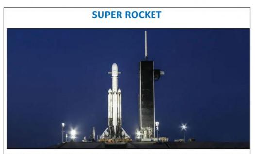
Falcon Heavy is the world's most powerful rocket. It was first launched into space on February 6, 2018 and has been launched two more times since then. Falcon Heavy is a rocket that stands 70 m tall and weighs 1,420,788 kg. Regarding its structure, the first stage has three parts, or cores, each with nine identical rocket engines, making 27 engines in all. Each core is a Falcon 9, an earlier
