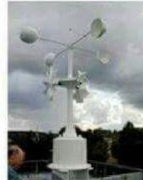
Anemometer (Wind speed)
