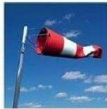
Wind sock (Speed and wind direction)
