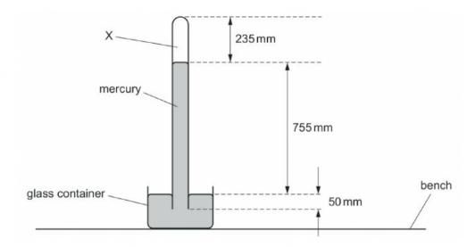
The total weight of the mercury barometer is 38 N. The area of the glass container in contact with the bench is  $200\,\mathrm{cm}^2$ .
