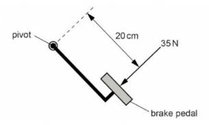
Calculate the moment of the force about the pivot. Include the unit.
