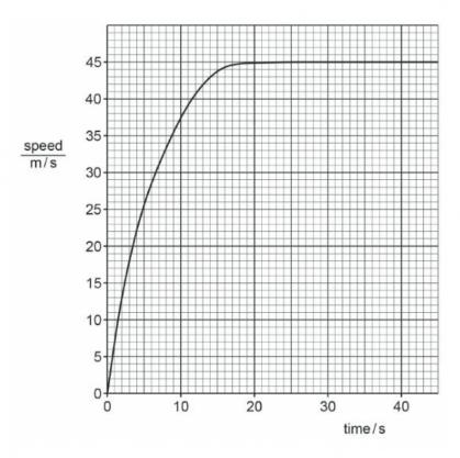
Calculate the distance the box moves between time = 30 s and time = 40 s.
