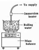
Some water in a container (as shown above) is brought to its boiling point by an immersion heater. A watch is then started and the time, t, to boil off a mass, m, of water is found. If the heater has a power, P, the specific latent heat of vaporisation is
