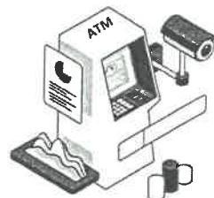
To increase security at cash machines, some banks have tried to make their ATMs a little smarter. They have added to the cash machine a small camera that looks directly into the eye of every customer. It scans one iris (the coloured part of the eye) and compares the tiny patterns of dots and other features to a code in its computer. If there is a match, the ATM will start counting out cash. If not, a message is automatically sent to the nearest police station.
