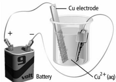
61. **Electroplating** Figure 27 shows a key being electroplated with copper in an electrolytic cell. Where does oxidation occur? Explain your answer.
