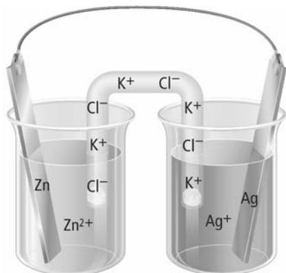
42. Figure 25 illustrates a voltaic cell consisting of a strip of zinc in a 1.0M solution of zinc nitrate and a strip of silver in a 1.0M solution of silver nitrate. Use the diagram and Table 1 to answer these questions.
