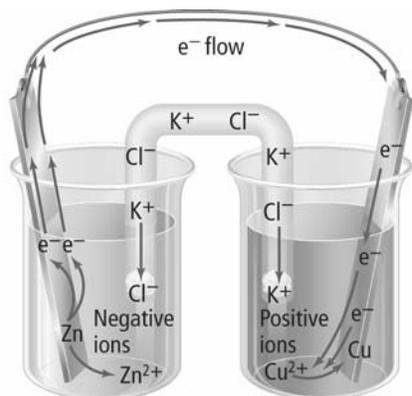
36. In **Figure 24**, identify the metal that is being oxidized. Identify the cathode.
