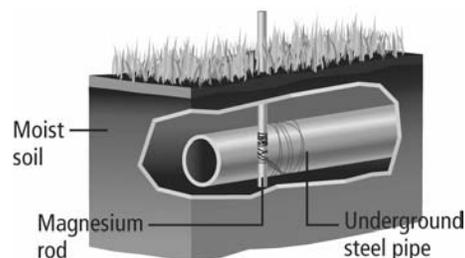
**74. Corrosion Prevention** Figure 29 shows how buried steel pipeline can be protected against corrosion. The steel pipe is connected to a more active metal that corrodes instead of the steel.
