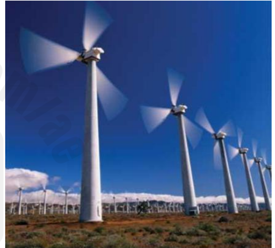
Figure 22 Wind energy is converted to electrical energy as a spinning propeller turns a generator.
