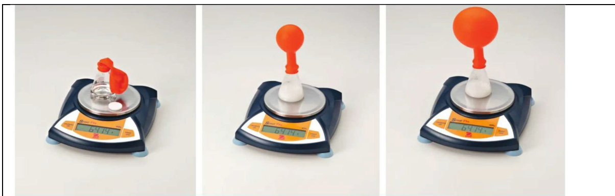
Figure 19 The reaction between sodium bicarbonate and hydrochloric acid produces carbon dioxide gas, which is collected in the balloon.
