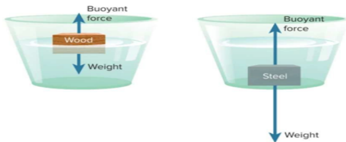
Figure 13 The steel block sinks because the buoyant force from the fluid is less than the gravitational force on the object. When the buoyant force is the same as or greater than the gravitational force—as with the wooden block—the object floats.
