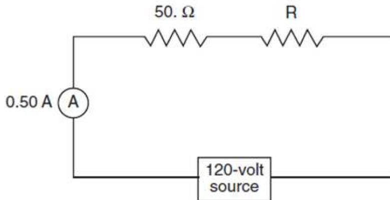
What is the equivalent resistance of the circuit?
