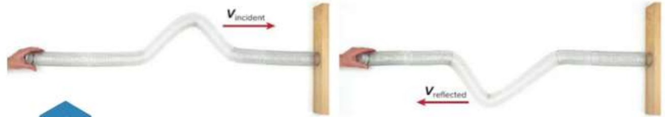
Figure 13 When a wave encounters a rigid boundary, the reflected wave is inverted. Note that the amplitude is not affected by the rigid boundary.
