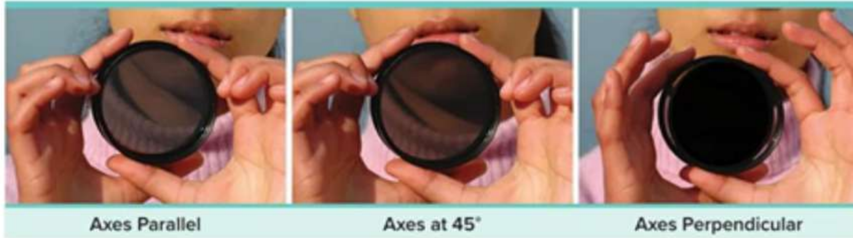
Figure 20 Polarizing filters with their axes parallel will allow the light with the same orientation to pass. With the polarizing axes at a 45° angle, the filters allow some light to pass. If the axes of the filters are perpendicular, the second filter will block the light that has passed through the first filter.
