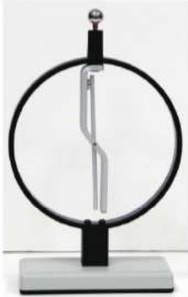
**FIGURE 1.8** A typical electrostatic demonstrator used in lecture demonstrations.
