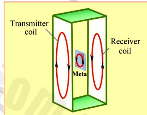
A current will be induced in the metal plate in the opposite direction and will tend to oppose the increase in the current in the transmitter coil. The increasing current in the metal plate will induce a current in the receiver coil that is in the opposite direction and tends to oppose the increase in the current in the metal plate (not shown in the diagram). Thus, the metal plate induces a current in the receiver coil that flows in the same direction as the current in the transmitter coil.
