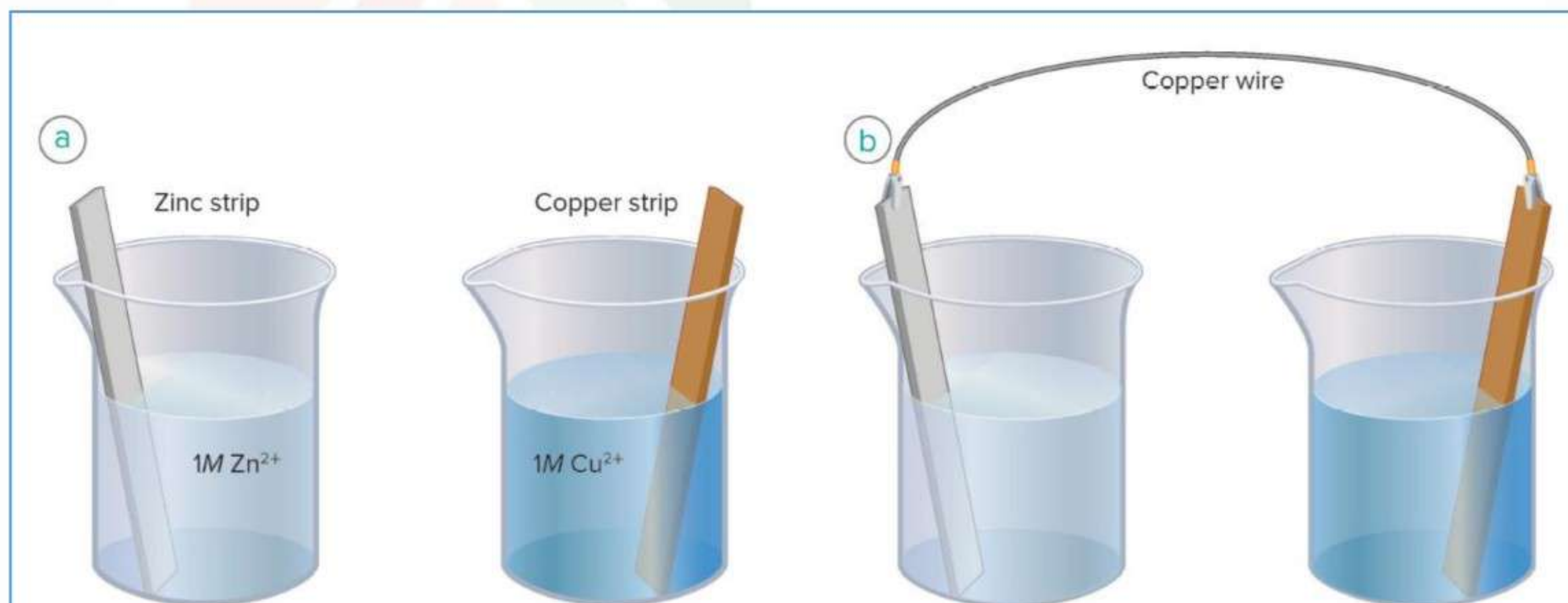
Figure 1 In a , zinc metal is immersed in 1M zinc sulfate solution, and copper metal in 1M copper(II) sulfate. In b , a wire joining the zinc and copper strips provides a pathway for the flow of electrons, but the pathway is not complete. Electron transfer is still not possible.
