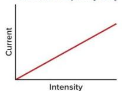
Current v. Intensity with Constant Frequency \geq f_0
