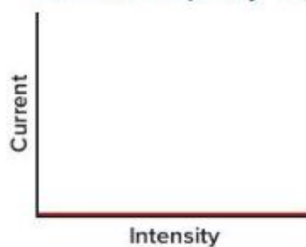
Current v. Intensity with Constant Frequency < f_0
