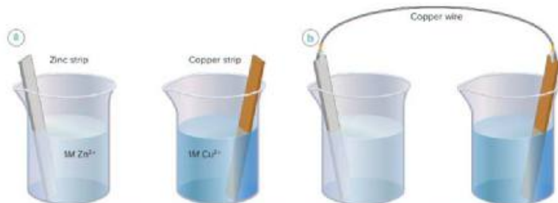
Figure 1 In a, zinc metal is immersed in 1M zinc sulfate solution, and copper metal in 1M copper(II) sulfate. In b, a wire joining the zinc and copper strips provides a pathway for the flow of electrons, but the pathway is not complete. Electron transfer is still not possible.
