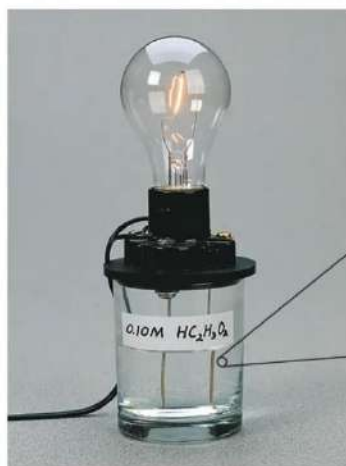
Figure 10 When electrodes are placed in 0.10M acetic acid solution, the light is dim. Compare this illustration with Figure 9 . Explain the difference in the brightness of the bulbs in terms of the concentration of ions in solution.
