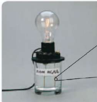
■ Figure 12 When electrodes are placed in 0.10M acetic acid solution, the light is dim. Compare this illustration with Figure 18.11 . Explain the difference in the brightness of the bulbs in terms of the concentration of ions in solution.
