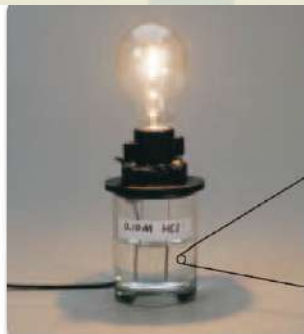
■ Figure 11 The light glows brightly when electrodes are placed in 0.10M hydrochloric acid solution because all of the HCl is in the form of hydronium ions and chloride ions.
