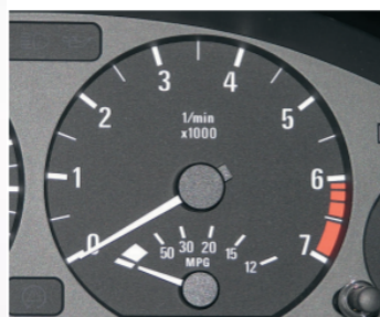
FIGURE 9.9 The tachometer of a car measures the frequency (in cycles per minute) of revolutions of the engine.
