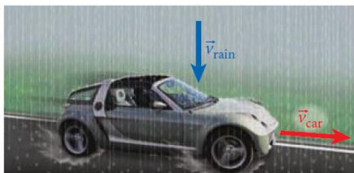
FIGURE 3.20 The velocity vectors of a moving car and of rain falling straight down on the car, as viewed by a stationary observer.
