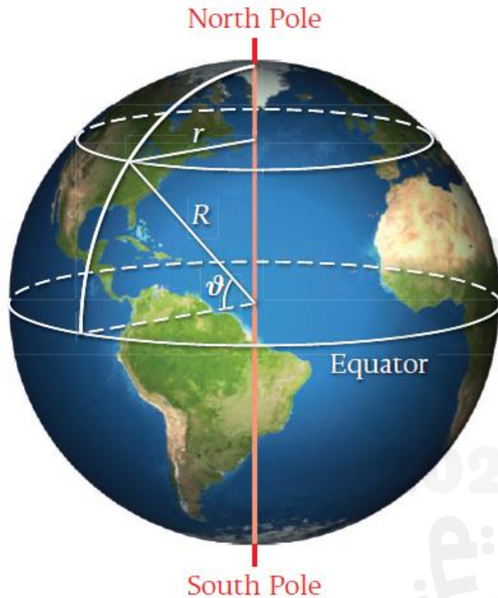
FIGURE 9.11 Earth's rotation axis is indicated by the vertical line. Points at different latitudes on the Earth's surface move at different speeds.
