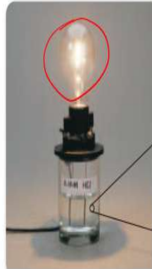
Figure 11 The light glows brightly when electrodes are placed in 0.10M hydrochloric acid solution because all of the HCl is in the form of hydronium ions and chloride ions.
