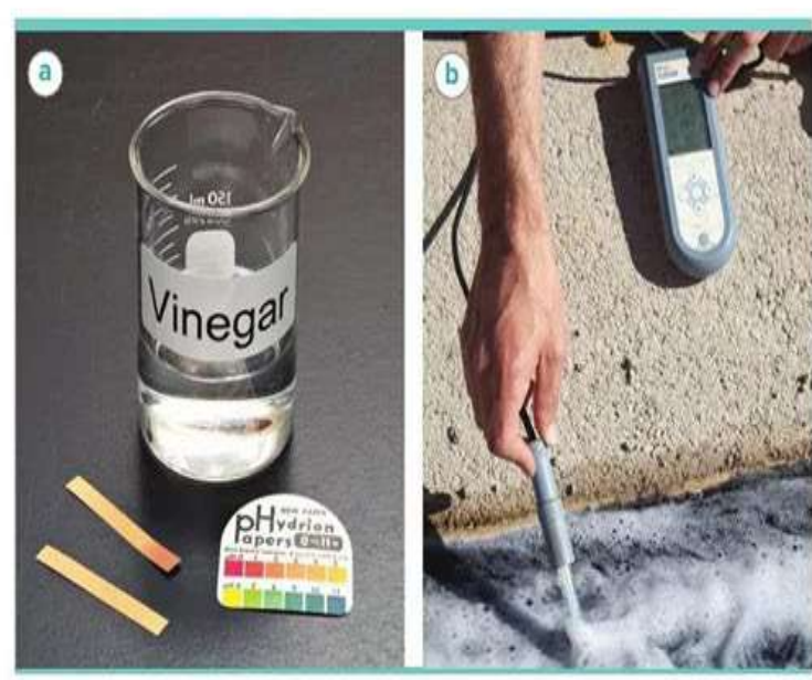
Figure 16 The approximate pH of a solution can be obtained by wetting a piece of pH paper with the solution and comparing the color of the wet paper with a set of standard colors as shown in a . The portable pH meter in b , which is being used to measure the pH of rain water, provides a more accurate measurement in the form of a digital display of the pH.
