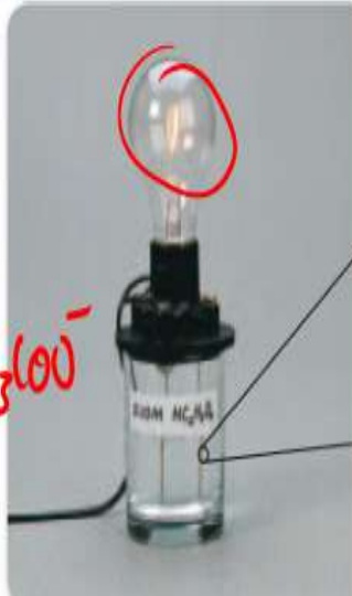
Figure 12 When electrodes are placed in 0.10M acetic acid solution, the light is dim. Compare this illustration with Figure 18.11. Explain the difference in the brightness of the bulbs in terms of the concentration of ions in solution.
