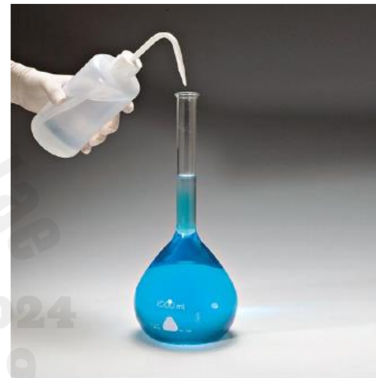
Step 3: Distilled water is added to the flask to bring the solution level up to the calibration mark.
