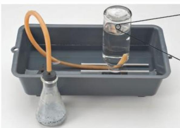
**Figure 8** In the flask, sulfuric acid ( $H_2SO_4$ ) reacts with zinc to produce hydrogen gas. The hydrogen is collected at 20°C.
