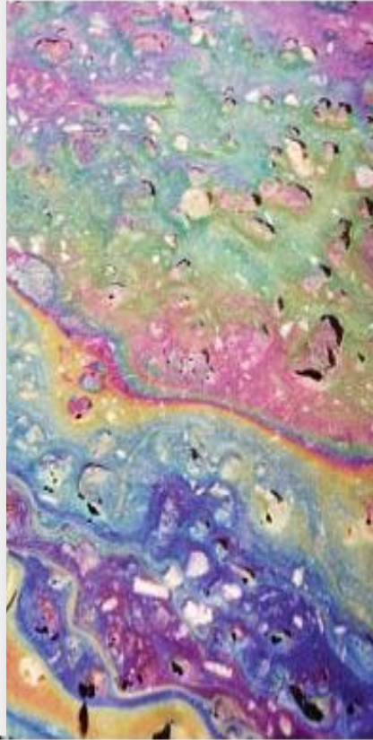
Figure 8 At soap film thicknesses of \lambda/4 , 3\lambda/4 , 5\lambda/4 , etc., light with wavelength \lambda is in phase. Bands of that color light are visible at those thicknesses.
