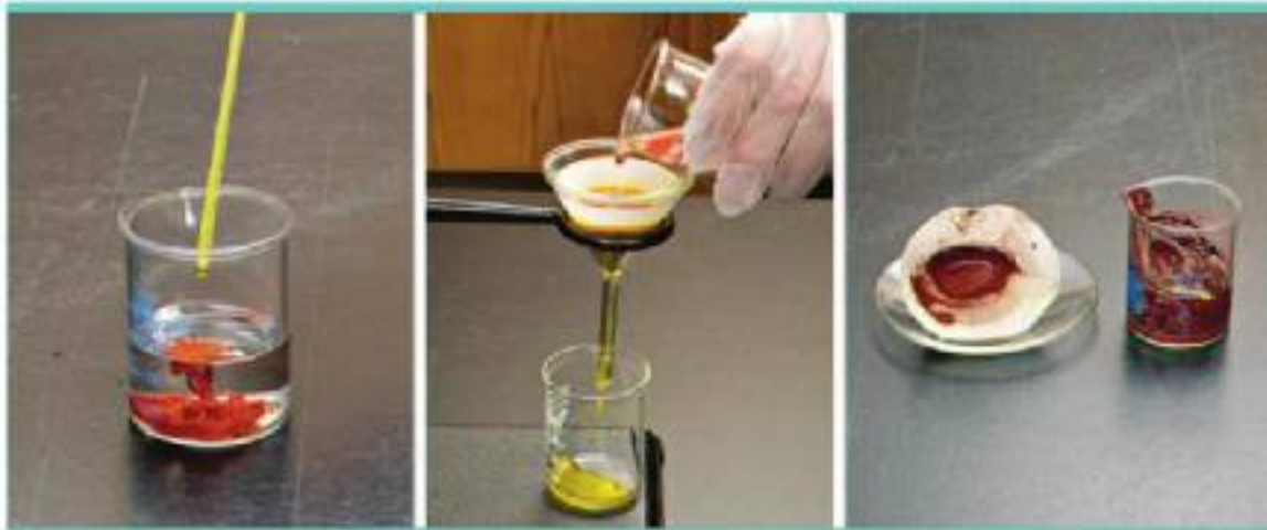
Figure 8 Silver chromate is formed when potassium chromate is added to silver nitrate. Note that not all of the precipitate can be removed from the filter paper. Still more of the precipitate is lost because it adheres to the sides of the beaker.
