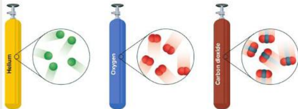
Figure 5 Gas tanks of equal volume that are at the same pressure and temperature contain equal numbers of gas particles, regardless of which gas they contain.
