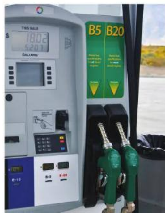
Figure 7 B20 is 20% by volume biodiesel and 80% by volume petroleum diesel. Biodiesel is a clean-burning alternative fuel that can be produced from renewable resources, such as vegetable oil.
