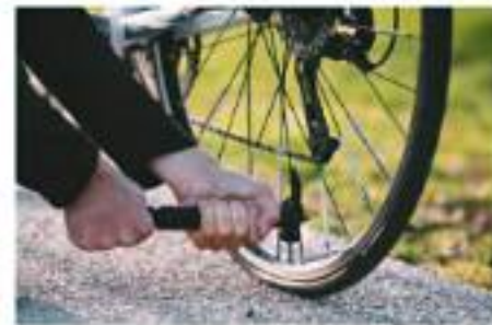
Figure 6 The volume and temperature of this tire stay the same as air is added. However, the pressure in the tire increases as the amount of air present increases.
