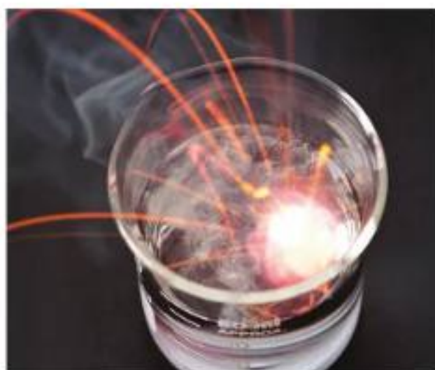
Figure 3 Potassium metal reacts vigorously with water, releasing so much heat that the hydrogen gas formed in the reaction catches fire.
