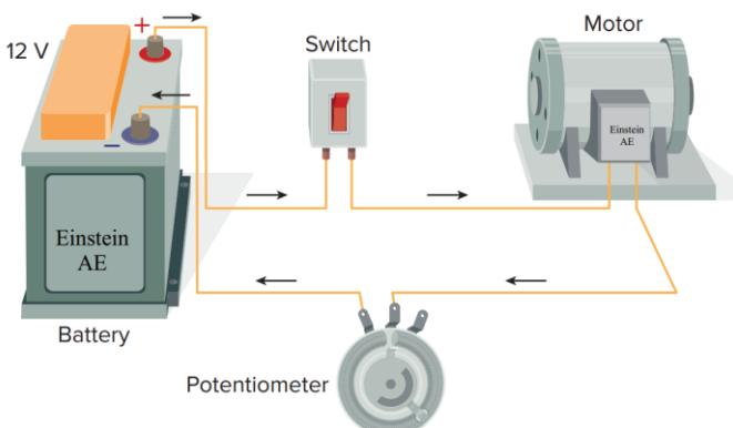
A. How can you change the **speed of rotation** of the motor **without adding or removing any components** from the circuit?
