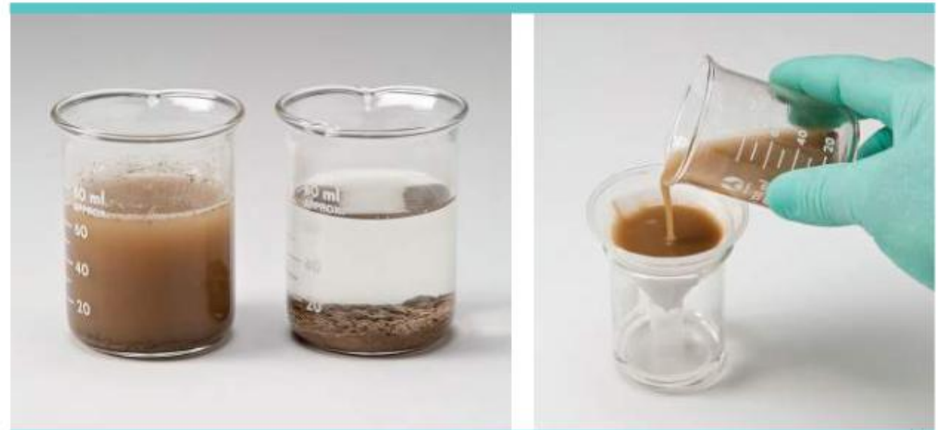
Figure 1 A suspension can be separated by allowing it to sit for a period of time. A liquid suspension can also be separated by pouring it through a filter.
